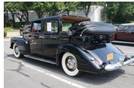
This is the only 1941 Cadillac Towncar-Landaulet ever made. It is built exactly like the custom body cars of the 1930's, with a wooden frame, over which was placed the aluminum body sheet metal. The only standard Cadillac parts used were the front and rear bumper, grill, front fenders and hood. The cowl and rear fenders are standard 1941 Cadillac but with significant modification. The current owner possesses a copy of the complete file from Derham Body Company in Rosemont PA for this automobile.
