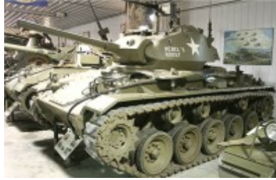
M24 with twin Cadillac V8 engines and Hydra-matic transmission
