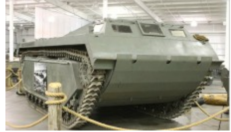
LVT(3) (Landing Vehicle, Tracked) one of 2,962 built for US Marine Corps. Powered by two Cadillac V-8s
